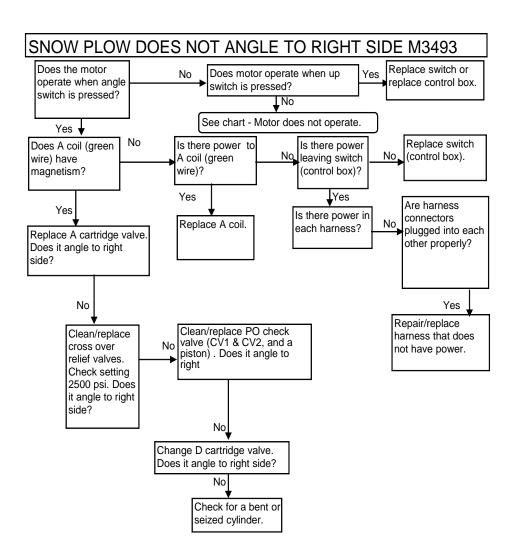
Note: Before start troubleshooting check that plow moves up and down. If plow does not move up and down see "plow does not raise".
